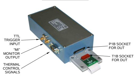
The externally-generated TTL trigger signal must be applied to the SMA connector shown above. The input impedance is 50 Ohms.
